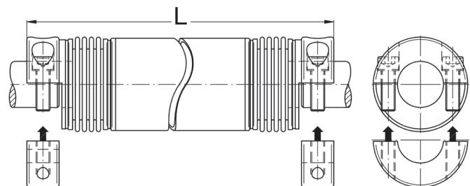
**Caution:** Since the metal bellows are made of thin stainless steel, particular care is required in handling. Deformations of the bellows can impair the function.
